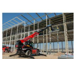
Exceptional ground clearance Optimum stability on stabilisers with a ground clearance of 43 cm under wheels.
